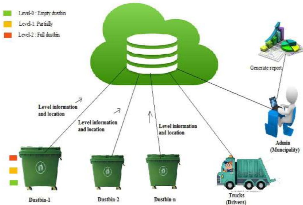
Fig.6 working structure of system
